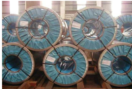
Thin & Clean Steel Sheet (0.3mm to 2.5mm thick)
