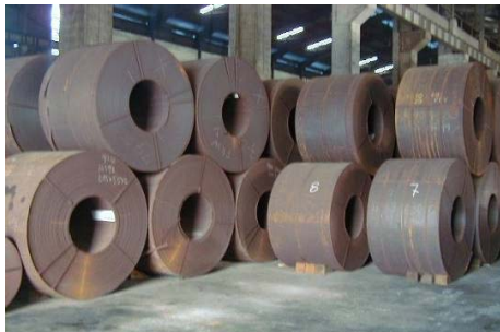
Thick & Rusty Steel Sheet (1.7mm to 3.5mm thick)
